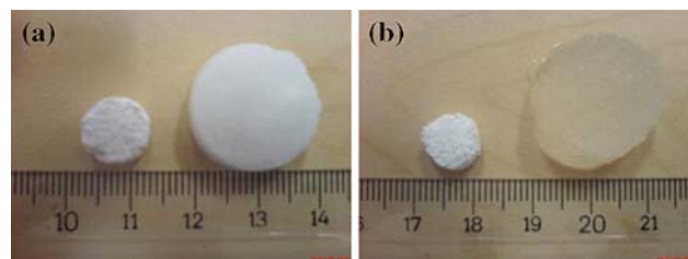
Fig. 3 Photographs of (a) SPHC in dried (left) and swollen state (right), (b) SPH in dried (left) and swollen state (right)
